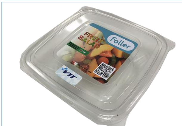
Figure 11. Printed food freshness sensor from VTT, communicating through RFID link.
