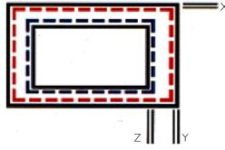
Seal Ring -Lid OD and Preform OD - - - -Preform ID \_ \_ \_ \_
