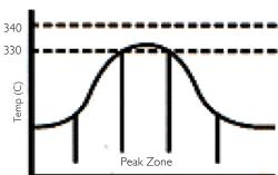
Rise Rate: 25° - 75° C Per Minute Peak Zone: 330° - 340° C 2-5 minutes Above 280° C Cool Rate: 25° - 50° C Per Minute Atmosphere: Hydrogen and/or Nitrogen
