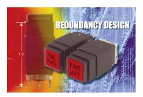
Electro-Mech has introduced its Series 644-2100 compact quad lamp / LED pushbutton switch assembly. It mounts in a 0.698 square mounting hole and accomodates up to four T-1 sub midget flange based lamps or LED's for maximum brightness or lamp redundancy. With circuitry up to 2PDT, this switch offers maximum display versatility in a compact package.
