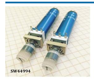
Electro-Mech has introduced its SW44994 pot. + switch assembly with both rotary and push-on / pull-off switch functionality for maximum operational control. The SPDT-DPDT device offers a rotary potentiometer with 10K-ohm resistance, a D-flat shaft, and push/pull mechanism. Assembly includes solder lug terminals (PC pins are also available) and requires 2.03 behind panel depth. Edgelit knob is sold separately.
