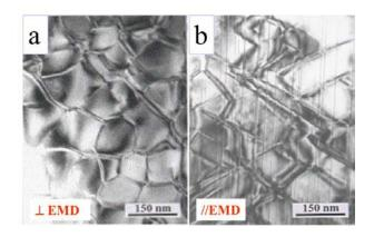
Cellular microstructure of Sm<sub>2</sub>Co<sub>17</sub> type magnets
