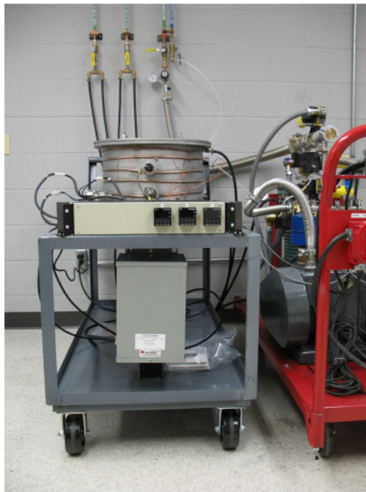
Figure 6: Front view of the vacuum system for thermal stability studies
