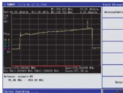
The field strength measurement automatically takes into the account of the antenna factor. The antenna table is definable by the standard N9340B PC software.
