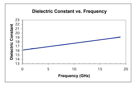
\* - Data obtained from measurements on ring resonators. Metallization is co- fired 903-A silver.
