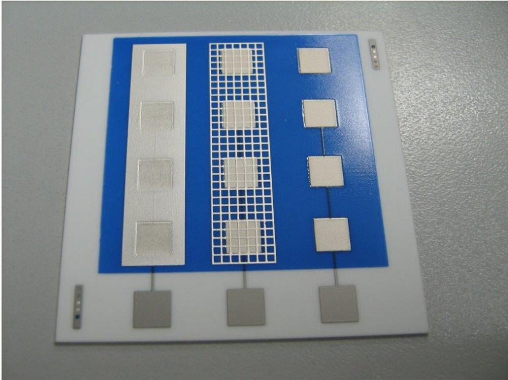
Figure 3 First top conductor (solid block to the left and hashing in the middle) – layer 5
