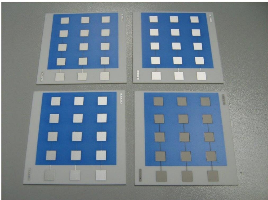
Figure 2 Dielectric layer (layers 2 and 4) superimposed on the first layer
