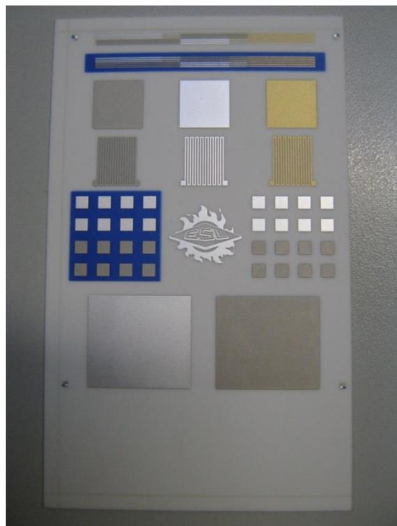
Figure 6 Mixed metal test pattern
