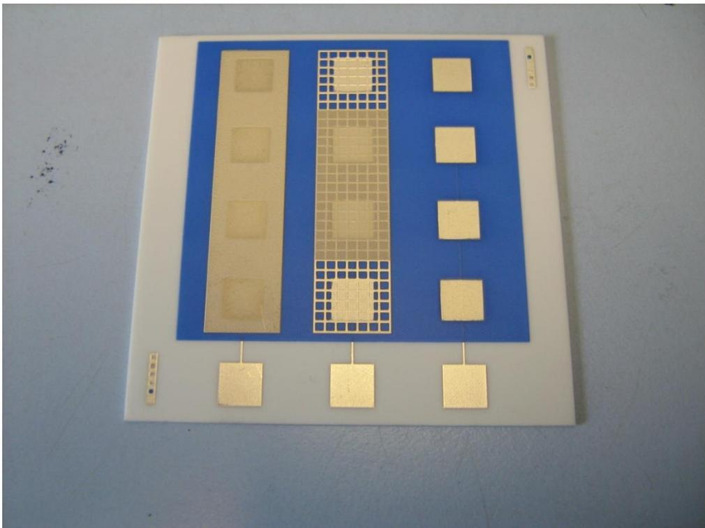
Figure 4 Second top conductor (solid block added to the centre hashed conductor) – layer 6
