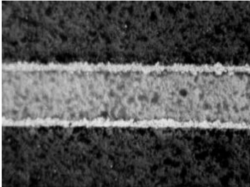
Figure 5. SEM of K-100 tape buried in 111-CF tape
