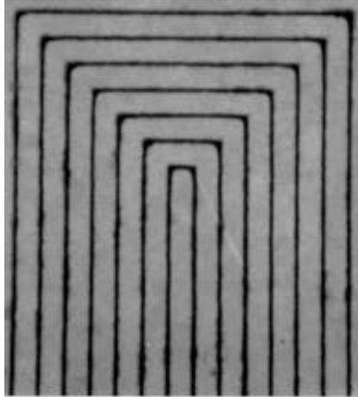
Figure 7. SEM of photoimaged Ag conductor (8 $\mu\text{m}$  lines on 50 $\mu\text{m}$  pitch)
