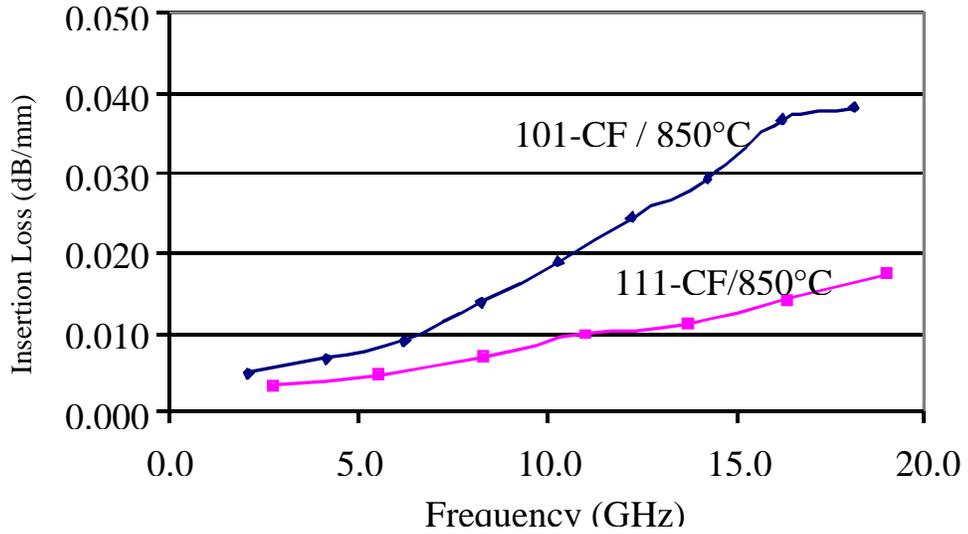
Figure 3. Loss versus frequency of 111-CF and 101-CF
