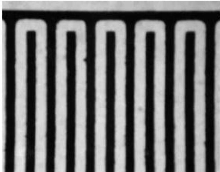
Figure 6. SEM of photoimaged electrode pattern (40 $\mu\text{m}$  lines, 60 $\mu\text{m}$  spaces)
