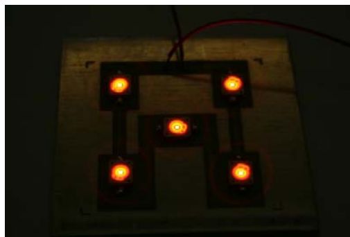
Figure 7 Glass based dielectric systems working at low voltage
