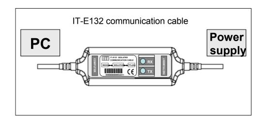
Note: It will not work if you connect the DB9 interface connector of the power supply to the RS232 interface connector of computer directly by a standard RS232 cable. Please use IT-E132 to connect them.
