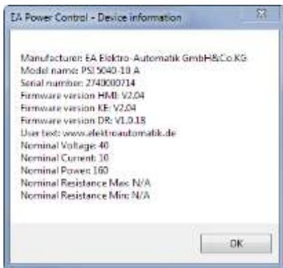
In the example with a PSI 5000 series power supply it becomes clear, that this device does not feature resistance mode (R mode). You can also see that the unit has no user text assigned (yet). The user text is intended to be used to distinguish multiple identical devices.
