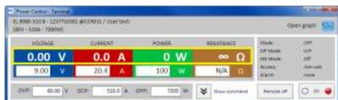
Similar to the value coloring on the devices with color TFT display, the actual values are separated from each other. In the single fields, they are located at the top (big digits). The colored area always shows at least three actual values. With electronic loads, it also shows actual resistance.
