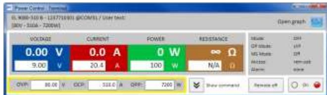
The allowed value range per input box is identical to what the device allows to adjust on the front panel for manual use. The adjustment range of a protection threshold always is 0...110% of the related nominal value. In case, any value you enter is too high or too low, it is not accepted and the former value will be displayed again.
