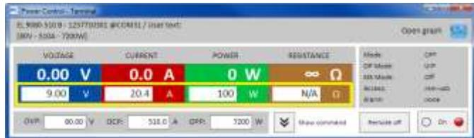
The allowed range of value per input box is identical to what the device allows on the front panel for manual use. The adjustment range of a set value is by default 0...102%, which can be narrowed by the so-called adjustment limits (here short: Limits). These can be defined manually in the MENU of the device or via **EA Power Control** in app "Settings". In case, any value you enter is too high or too low, it is not accepted and the former value will be displayed again.
