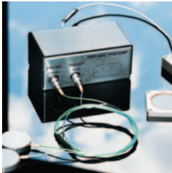
Capacitive sensor that can measure displacements smaller than a nanometer from Queensgate
