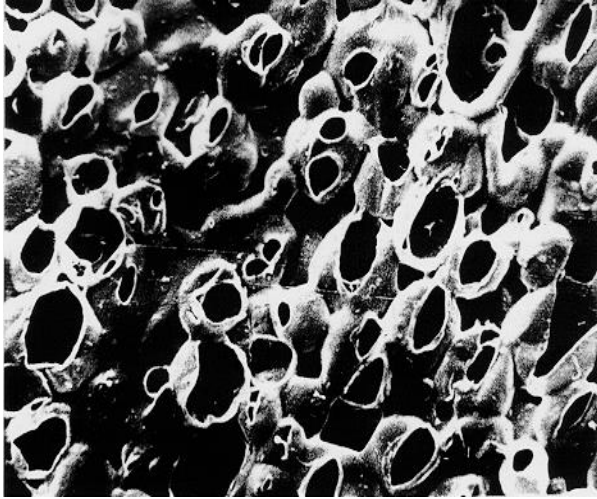
Fig. 16: Magnification of a separator, scale 500: 1 [3]
