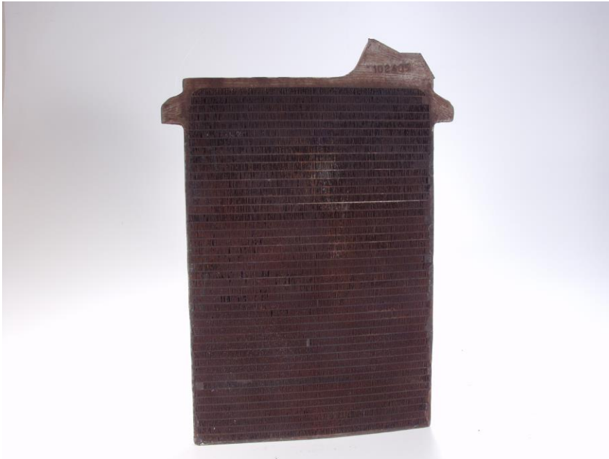
Fig. 10: Formed positive Planté plate
