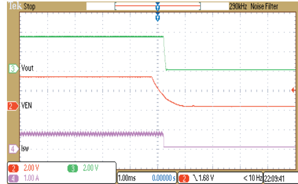
Shut Down ( I_{out} 1A \rightarrow Shut down)
