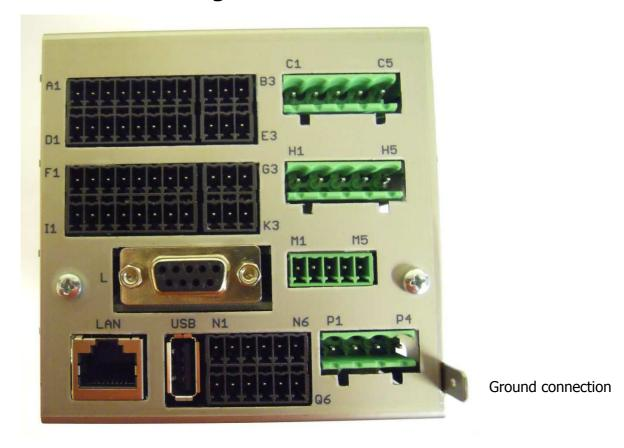
Ground connection (flat plug 6,3mm) must be connected to an earth rail via a thick cable (>=4qmm) in the shortest possible way (<20cm)!
