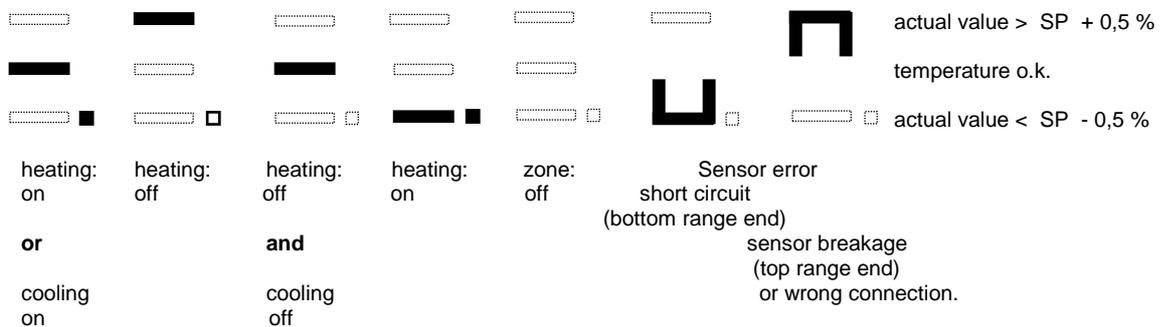
The flashing dec.-point shows, that either „heating“- or „cooling“-output is active.
