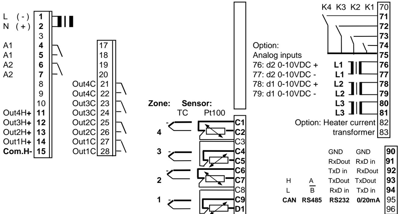
It is not permitted to connect the grounds of the sensor-inputs and bist. voltage-outputs with each other.
