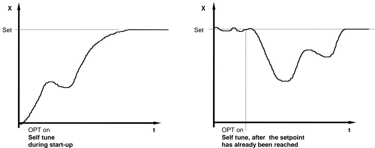
Self-tuning can be stopped by selecting the option **OPT = OFF** and pressing the „E“ - key.
