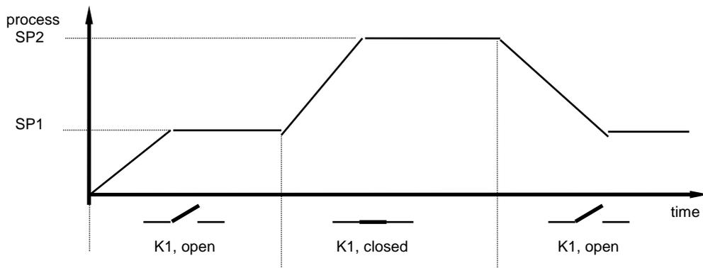
**A1 Alarm value 1, switching point**                      **Temperature monitoring: alarm value adjustment**
