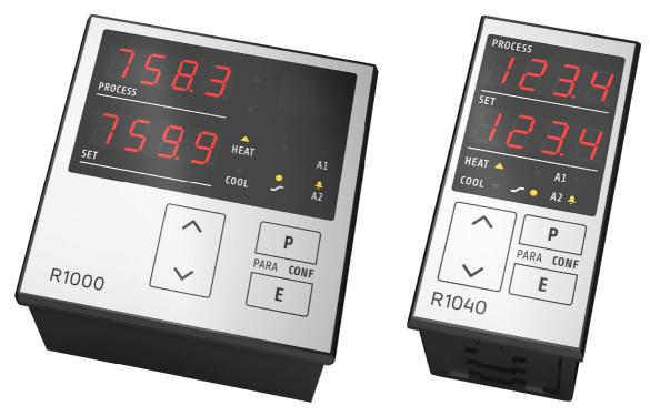
Installation depth: 60mm DIN-Format: 96mm x 96mm / 48mm x 96mm / 96mm x 48mm
