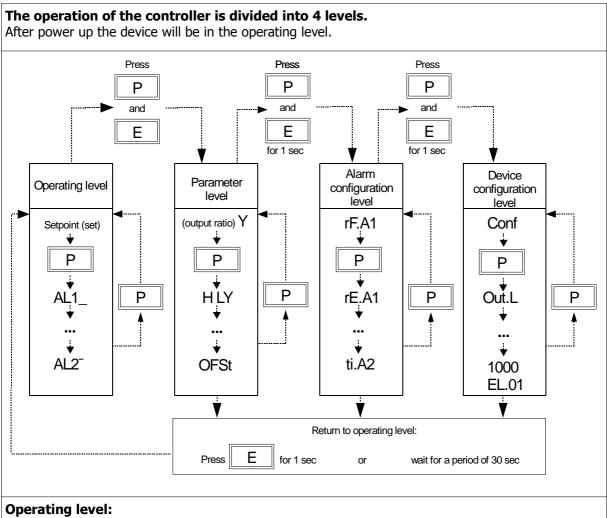
Process- and Setpoint value will be displayed simultaneously.
