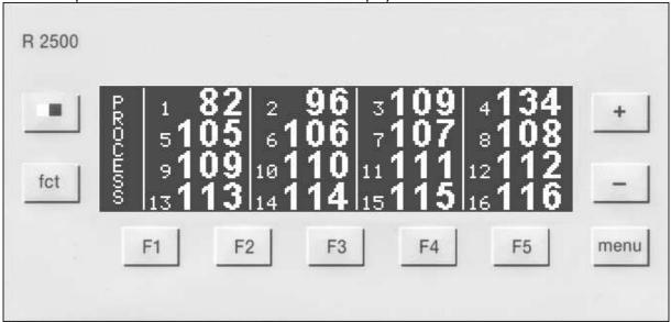
The device is operated by menus. The different parameters are displayed mainly in clear and can be displayed in various languages.
