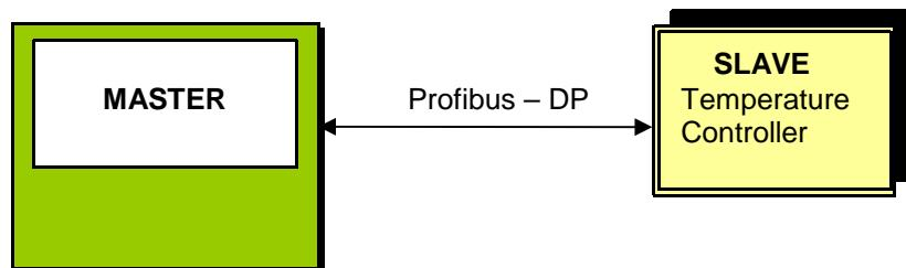
The PROFIBUS -interface allows the slave to be monitored and controlled by a PROFIBUS master. The data transfer between the slave and master takes place with the aid of the PROFIBUS-DP-protocol acc. to EN 50170.
