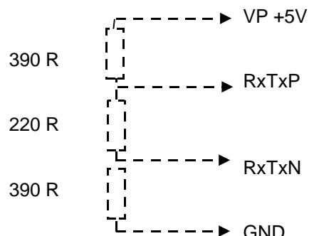
Termination resistors are integrated in the standard Sub-D9 Profibusconnectors.
