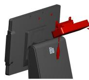
Remove the mounting screw covers from the back of the display and attach the VFD using the two screws included with the kit.
