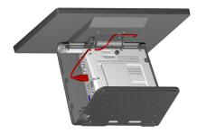
Route the USB cable through the cable clips as shown to connect the cable to the computer.
