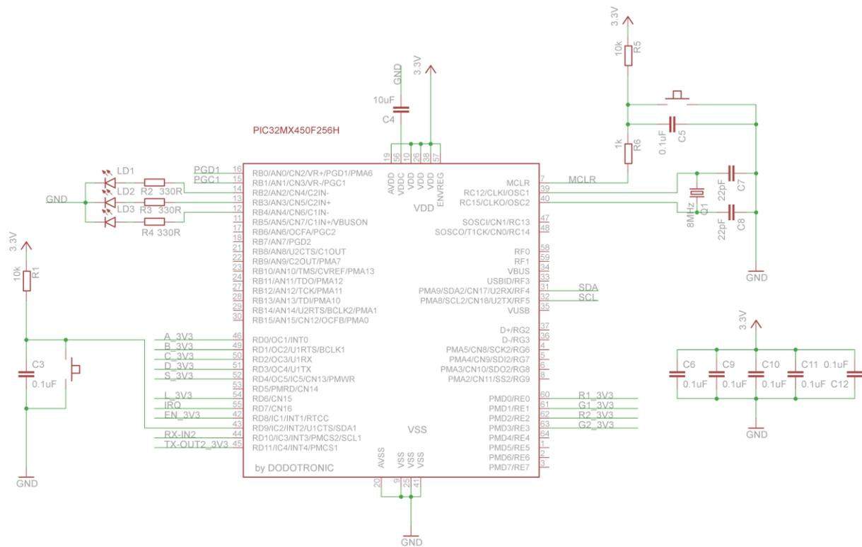
A fairly standard PIC32 microcontroller layout. Reset is provided via pulling MCLR to ground, and B1 pull RD9 to ground. B1 is used to trigger the bootloader. Hold it down while pressing the reset button.
