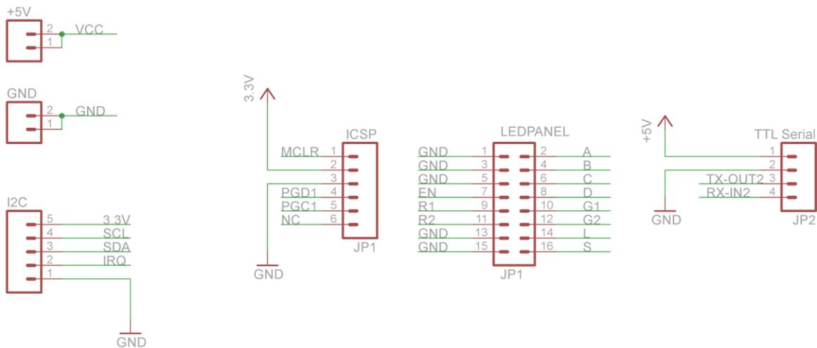
The LED panel connection follows the HUB08 standard connection for LED matrix display panels. ICSP allows for in circuit (non bootloader) programming normally only required for initial program
