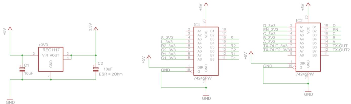
Since the microcontroller runs at 3.3V, we must convert the 5V the board runs at via a regulator. While most LED panels contain buffers and will probably run just fine being controlled at 3.3V, we use buffers to maintain 5V outputs and prevent load on the microcontroller. This also gives us a proper 5V TTL serial connection (the microcontroller will happily accept 5V input, and the 74HC245 gives us 5V output).
