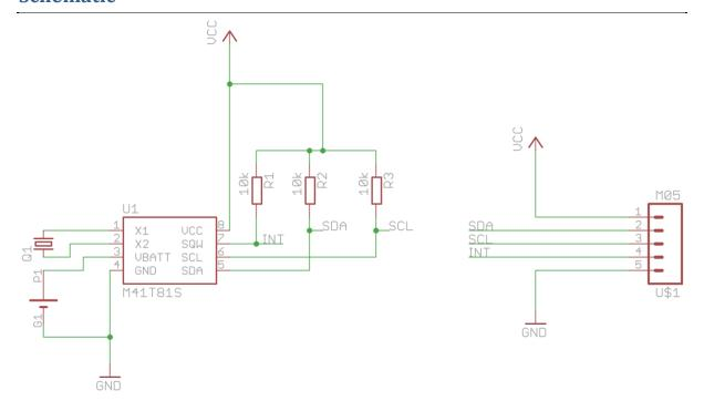
The MOD-1005 schematic is pretty straightforward. Don't forget to have a look at the M41T81S datasheet so you know how to get the most out of the RTC.
