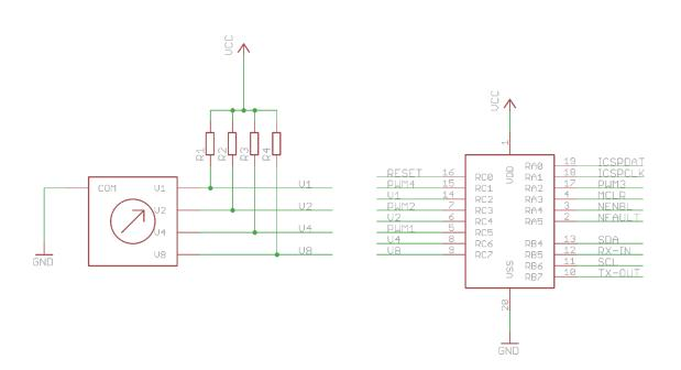
The I2C Address Selector drives pull-up resistors low. A PIC16F1509 microntroller is used to output multiple PWM connections at the same time while also communicating over I2C and TTL Serial.
