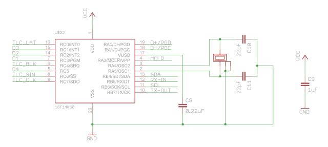
The PIC18F14K50 handles the interfaces with the outside world. It loads the TLC5926 for each digit and switches the digit using 9953 MOSFETs. Only one digit is actually active at any one time.
