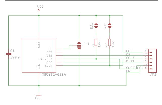
The MOD-1009 schematic is pretty straightforward. Don't forget to have a look at the MS5611 datasheet so you know how to get the most out of the pressure sensor.
