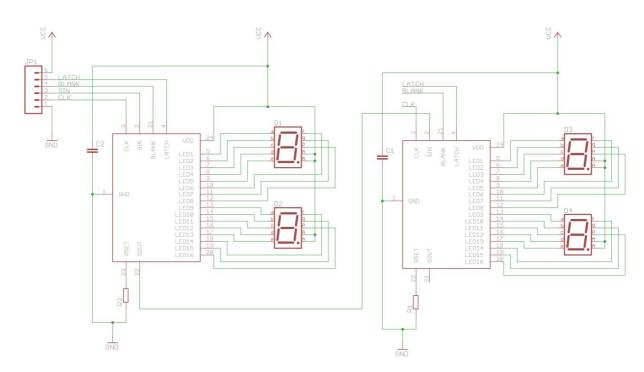
The DSP-7S04 module uses two CAT4016 chips to control 4 seven segment displays. The current setting resistor is chosen to supply approximately 20mA to each segment.
