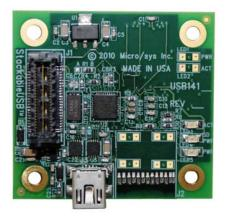
The USB1411 easily expands the solid state memory capacity of any StackableUSB Host computer or microcontroller. Designed for rugged embedded systems requiring secure connections, all memory devices are soldered to the module to increase shock and vibration tolerances. The module provides high-speed data transfers up to 30MB/s. The USB1411 comes as a 1GB or 2GB device, making it ideal for data logging and application programs.
