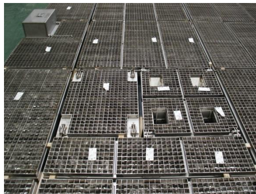
Trial-build assembly of Darflare™ heat shield before shipment to customer
