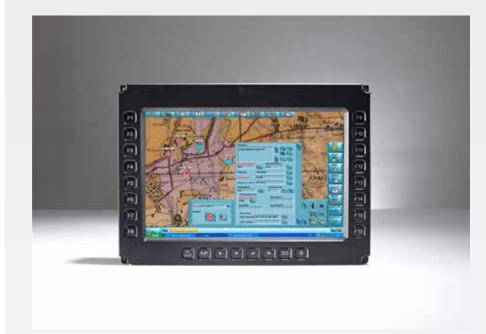
Esterline's TX-338 is an extremely rugged 15-inch wide-screen (1920x1200 pixels) display for the highly demanding environment of the utility vehicle, helicopter or ground army vehicle. The TX-338 offers an ideal solution for battlefield management, command and control, driver's view enhancement, reconnaissance or local situational awareness inside today's rugged vehicles.
