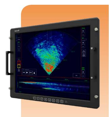
The RFD-454 is a Ruggedized 21,3" QXGA (2048 x 1536) high resolution display, designed and qualified for use in harsh environments such as airborne applications e.g. rotary wing.
