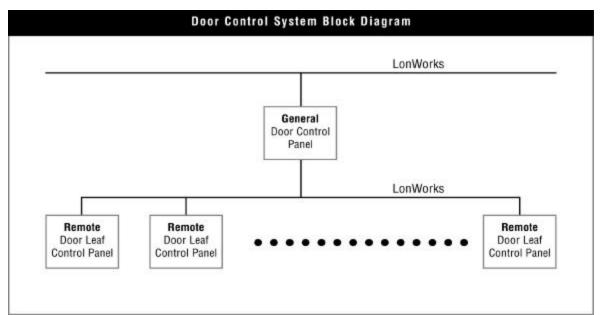
be accomplished through discrete signals or through the LonWorks network. With the use of LonWorks, for safety reasons, some of the discrete signals are also used to actuate the critical safety isolation relays.
