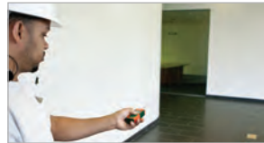
Laser distance meter with built-in tools to quickly calculate area even in hard-to-measure spots.
