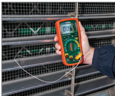
Verify Temperature output on HVAC units using Model EX355
