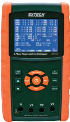
Model 382100 includes 1200A Clamp Probes
