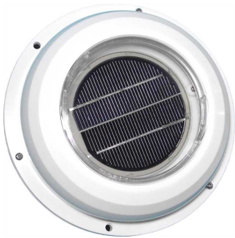
C-0702 ABS plastic cover Renew 20 m 3 of air per hour. Outer Diameter: 215 mm. Weight: 720 g.
