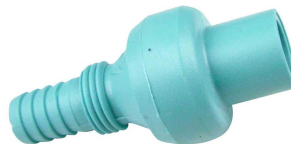
C-6012 Non-return valve For all immersion pumps. The direct connection to the pump outlet prevents back pressure. Hose Ø10 mm. Measurements: Length 50 mm Ø27 max.
