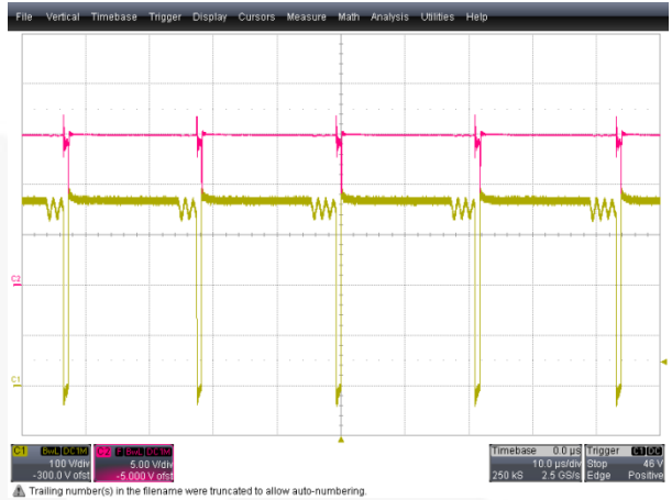
Figure 12. Full-Load Condition, 265 V AC (CH1: V DS (100 V/div), CH2: V CC (5 V/div), Time: 10 μs/div)
