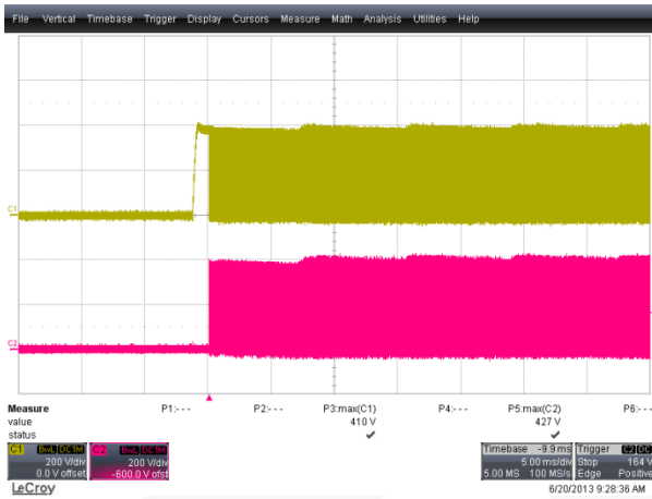
Figure 15. V_{DS}=410\text{ V} , V_{DIODE}=427\text{ V} , Startup Condition, Full-Load Condition, 265 V_{AC} , (CH1: V_{DS} (200 V/div), CH2: V_{DIODE} (200 V/div), Time: 5 ms/div)
