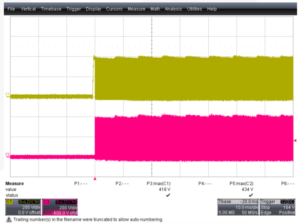
Figure 18. V_{DS}=416\text{ V} & V_{DIODE}=434\text{ V} , 3.3 V Output Short Condition, 15 V Full-Load Condition, 265 V_{AC} , (CH1: V_{DS} (200 V/div), CH2: V_{DIODE} (200 V/div), Time: 10 ms/div)
