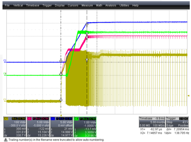
Figure 10. Startup Time=7.2 ms, 265 V AC , No-Load Condition (CH1: V DS (100 V/div), CH2: V CC (5 V/div), CH3: 15 V OUT (5V/div), CH4: 3.3 V OUT (1 V/div), Time: 5 ms/div)
