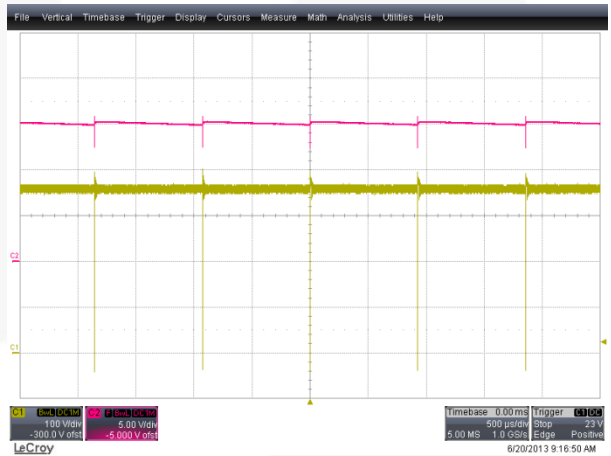
Figure 14. No-Load Condition, 265 V AC (CH1: V DS (100 V/div), CH2: V CC (5 V/div), Time: 500 μs/div)
