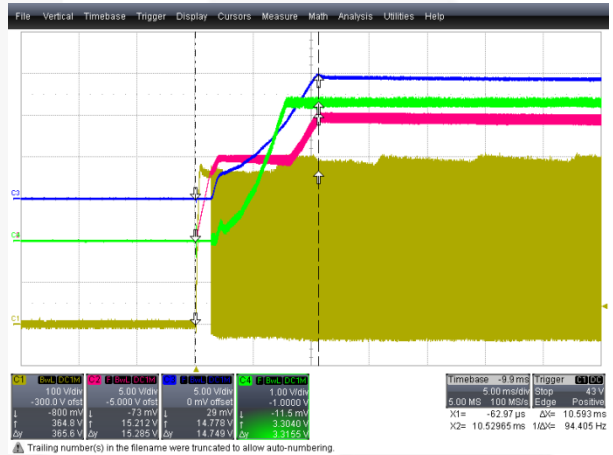
Figure 8. Startup Time=10.6 ms, 265 V AC , Full-Load Condition (CH1: V DS (100 V/div), CH2: V CC (5 V/div), CH3: 15 V OUT (5V/div), CH4: 3.3 V OUT (1 V/div), Time: 5 ms/div)
