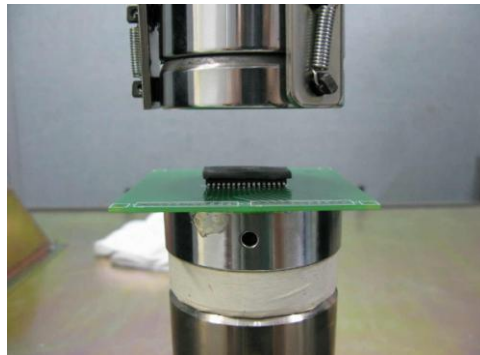
Figure 6. Compression Test with SPM package, PCB and 2mm T.I.M
