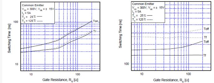
**Figure 19. Turn-On / Turn-Off Characteristics vs. Gate Resistance**
