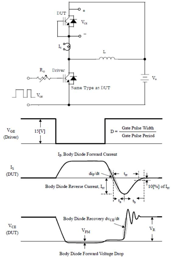
Figure 30. Diode Reverse Recovery Characteristics Test Circuit & Waveforms
