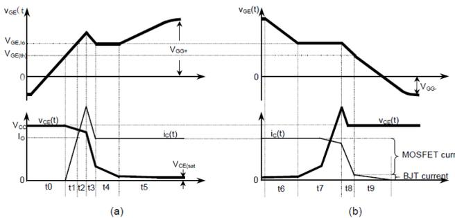
Figure 17.  $V_{GE}(t)$ ,  $V_{CE}(t)$ ,  $I_C(t)$  Switching Waveforms
