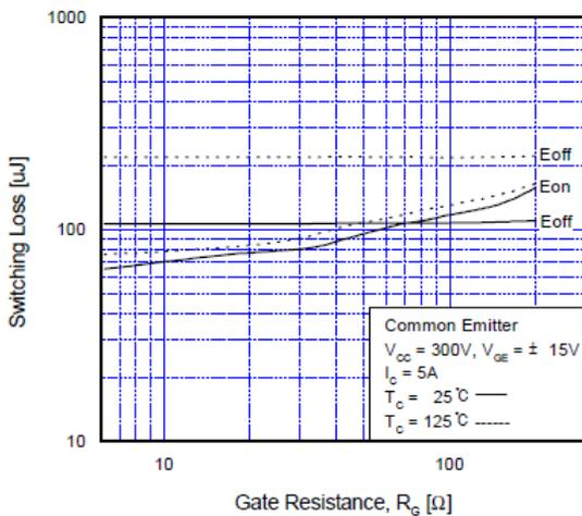
**Figure 21. Switching Loss vs. Gate Resistance**
