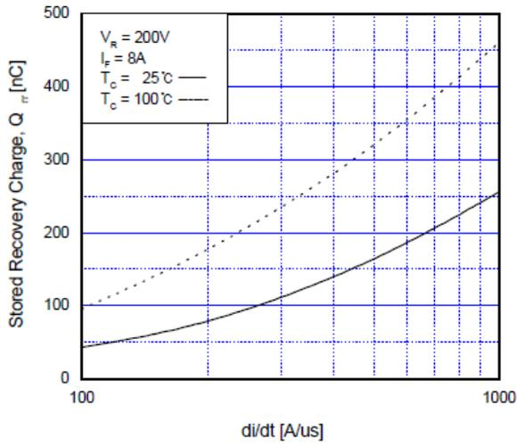
Figure 28.  $Q_{rr}$  Characteristics with Changes in Case Temperature,  $di_F/dt$
