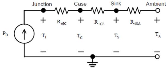
Figure 10. An Equivalent Circuit based on Thermal Resistances
