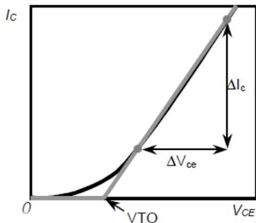
**Figure 9. Linear Interpolation of output characteristics at  $T_J = 150^\circ\text{C}$**
