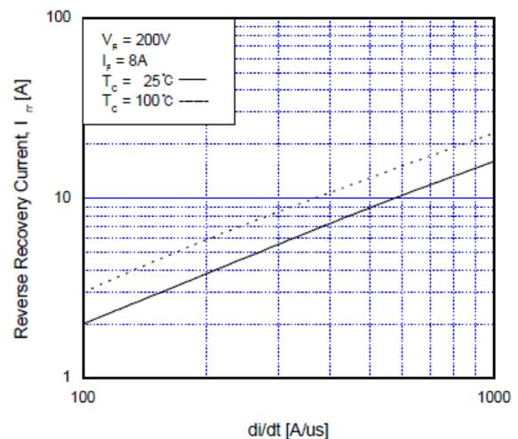
Figure 27. I<sub>rr</sub> Characteristics with Changes in Case Temperature, di<sub>F</sub>/dt
