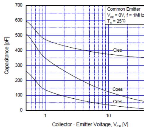
Figure 15. Capacitance Characteristics
