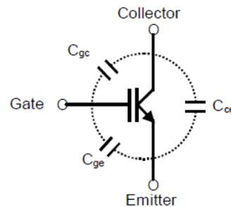
$$C_{ies} = C_{ge} + C_{gc}, C_{ce} \text{ is shorted}$$
