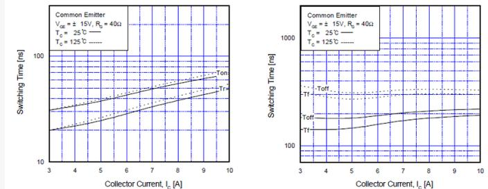
**Figure 20. Turn-On / Turn-Off Characteristics vs. Collector Current**
