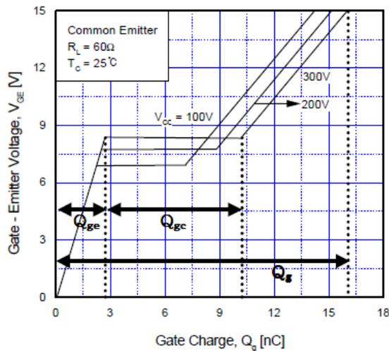
Figure 25. Gate Charge Characteristics by Vcc
