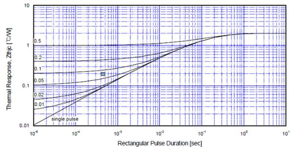
Figure 12. Transient Thermal Impedance of IGBT
