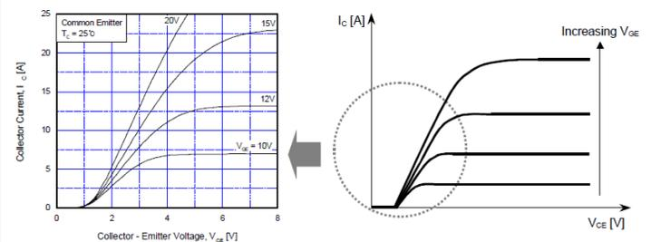
Figure 2. Static Characteristics of the IGBT
