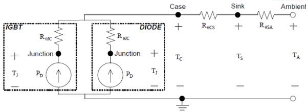
Figure 11. An Equivalent Circuit based on Thermal Resistances (co-pak)
