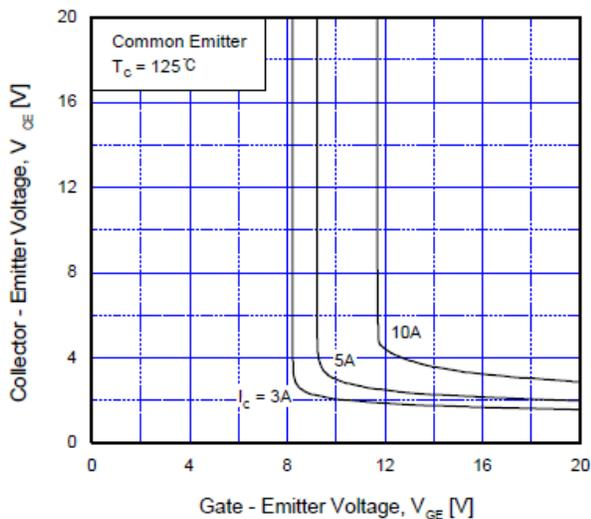
Figure 5. Saturation Voltage vs. V<sub>GE</sub> due to Collector Current, Case Temperature
