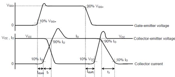
**Figure 18. The Switching Waveforms of Gate-Emitter Voltage, Collector-Emitter Voltage and Collector Current**
