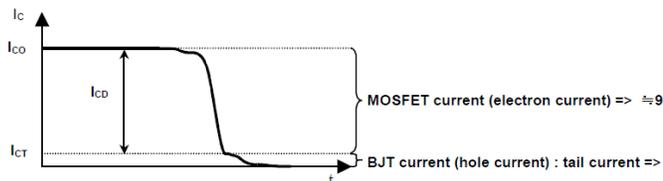
Figure 6. Collector Current during Turn-off
