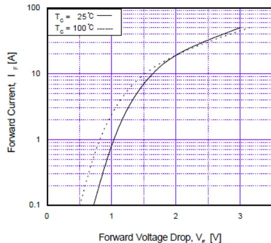
Figure 26. Forward Characteristics
