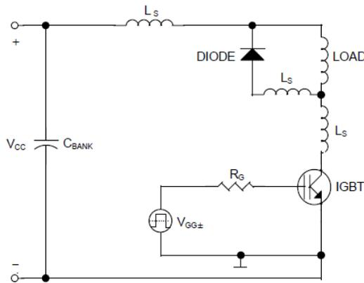
Figure 16. Diode-Clamped Inductive Load
