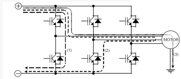
**Figure 23. Short Circuit Mode of IGBT**
