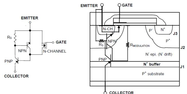
**Figure 1. Equivalent Circuit for the IGBT and a Cross Section of the IGBT Structure (PT and N-Channel)**
