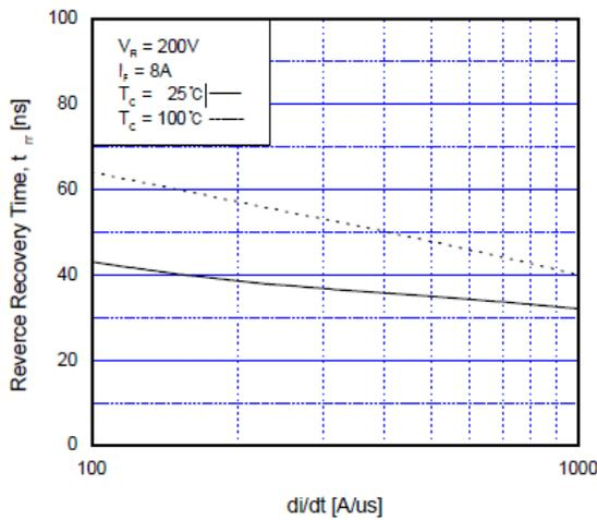
Figure 29.  $T_{rr}$  Characteristics with Changes in Case Temperature,  $di_F/dt$
