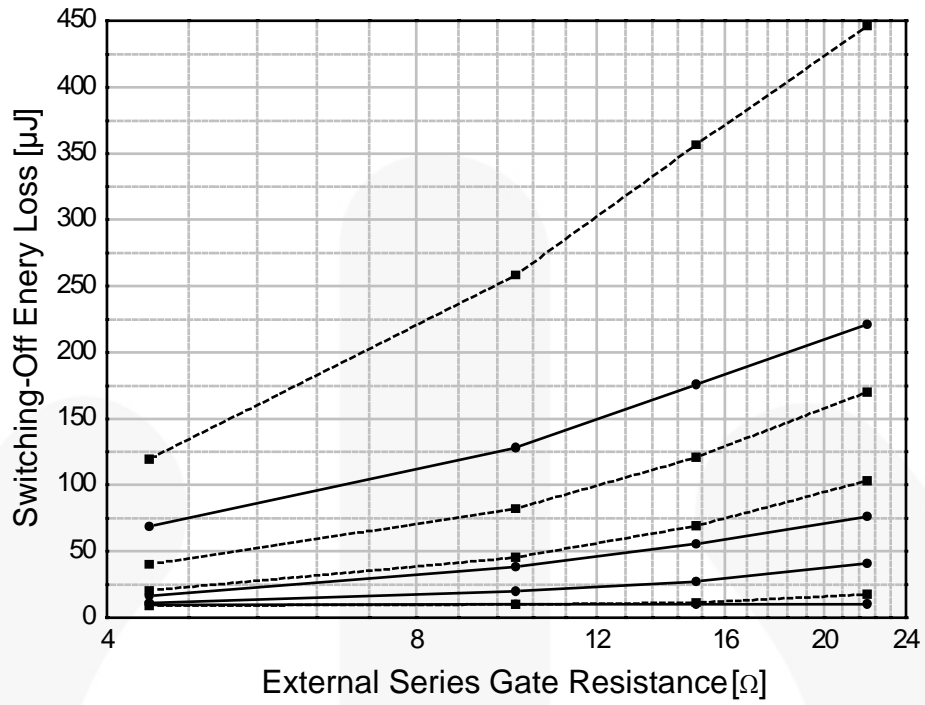
Figure 1. Energy Losses During Switching-Off Transition
