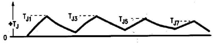
Figure 18. Equivalent Heat Input by Super-position of Power Pulses
