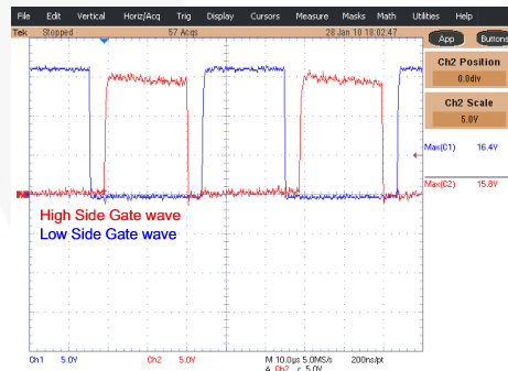
Figure 32. HVIC Gate Waveform
