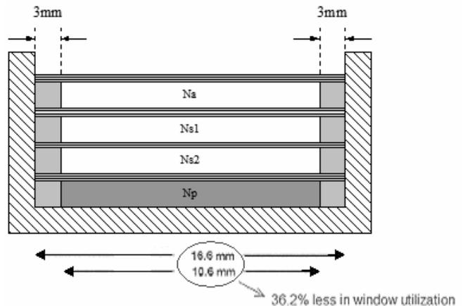
Figure 7. Window utilization for safety requirement.
