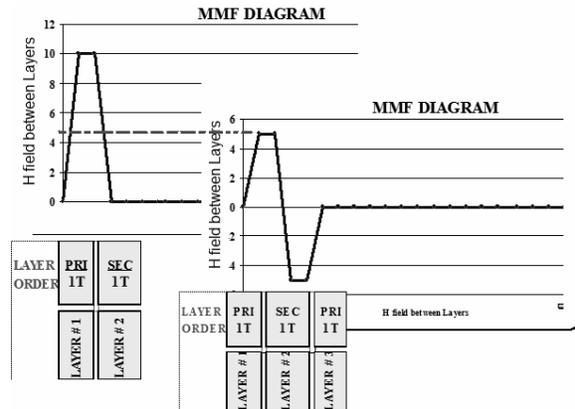
Figure 13. MMF diagram for layer arrangement.
