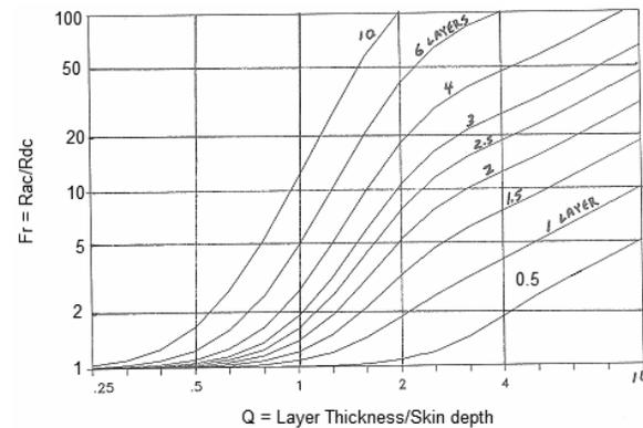
Figure 14. Dowell's equation in calculating AC resistance for different number of windings layer.
