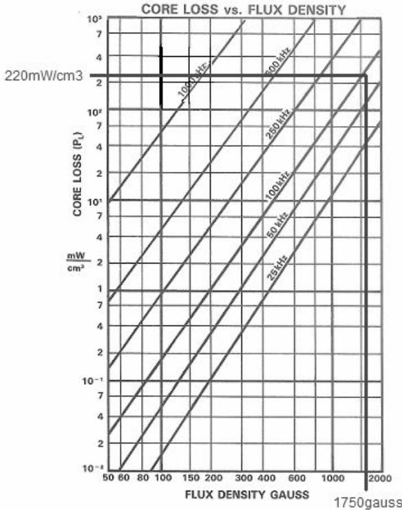
Figure 9. Core loss for any flux density at an operating frequency.
