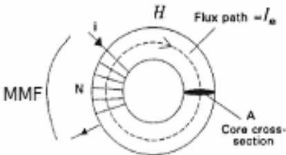
Figure 3. Example of a magnetic circuit.
