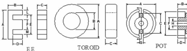
Figure 6. Different core shapes.
