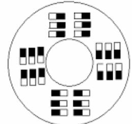
Figure 1. Individual magnets' alignment with and without external fields.
