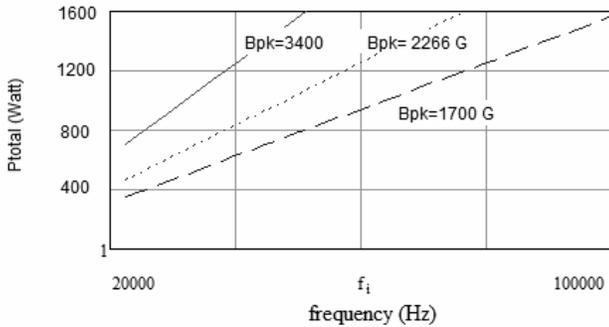
Figure 8. Effect of flux density in core power handling.
