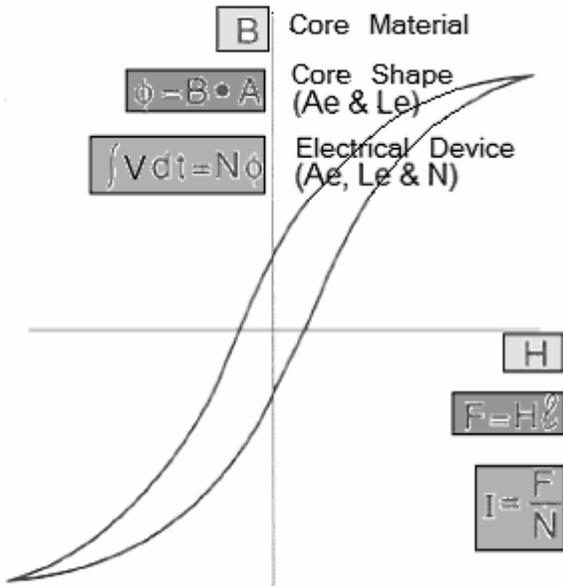
Figure 5. Transformation of material to electrical equivalent.
