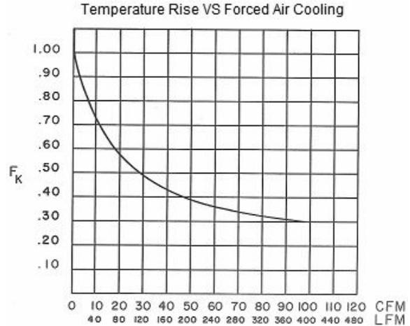
Figure 15. Cooling factor for different LFM and CFM assuming 0.25 ft<sup>2</sup> cross section for air flow.
