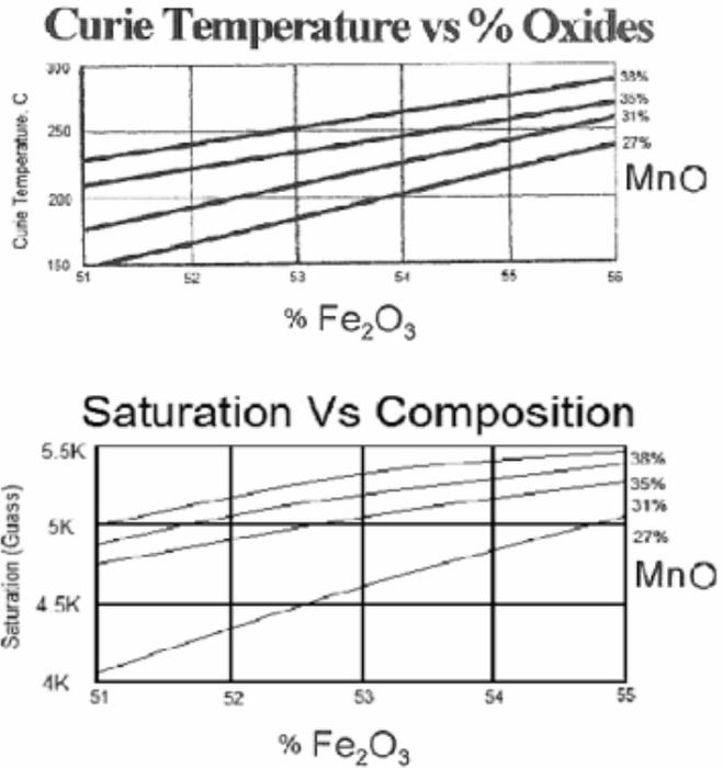
Figure 2. Effect of changing % of oxides and composition in material characteristic.
