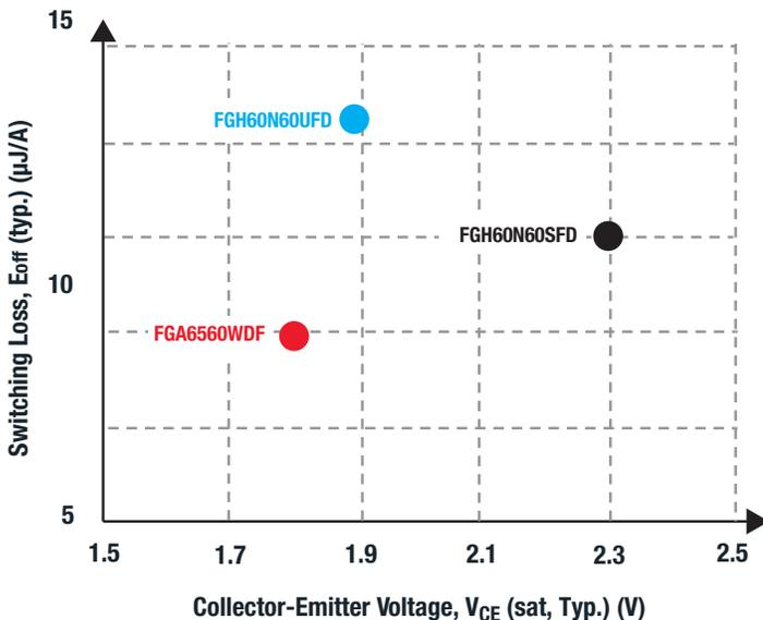
IGBT Power Loss Analysis on Welding Machine
