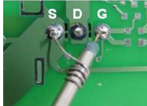
Figure 37. Measurement with Probe Tip and Ground Lead Removed
