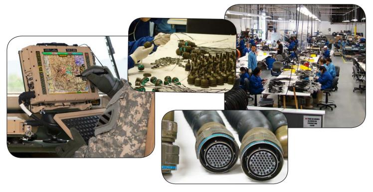
**Cable Design / Environments** considerations are carefully chosen in meeting Military vehicle requirements of temperature extremes, fuels, oil, chemical, shock, vibration, salt spray, and water submergence standards, as well as NBC and STB decontamination exposure.
