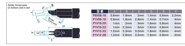
Shown above is a standard tip designed for use with 200W CROSS-HEATER. Other variations available include heater capacity-specific standard tips, many semi-custom tips and full custom tips.
