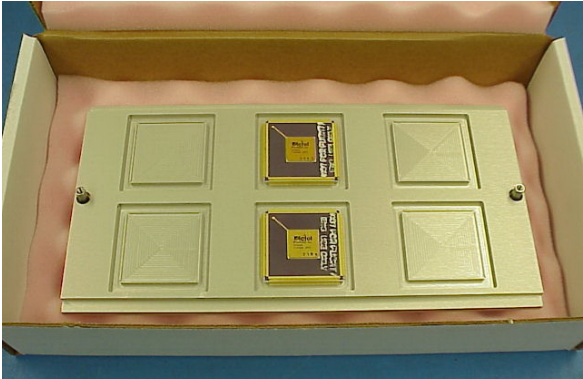
Photo of a 352 lead FPGA in a dedicated Fancort Matrix Tray:
