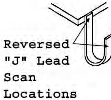
Figure 9-5. Scan Locations on Reversed J-Style lead
