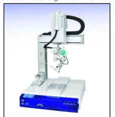
The UNIX-413S system includes solder position correction and can automate picking, component insertion, and soldering.
