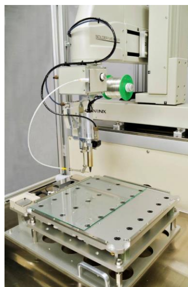
A UNIX 700S with an ultrasonic soldering unit installed
